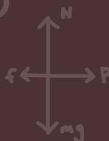
$$\begin{aligned} \Sigma F_x &= ma \\ P &= f = ma \\ \Sigma F_y &= ma \\ N - mg &= ma = 0 \end{aligned}$$
