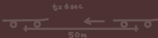
$$\vec{v} = \frac{d}{t} (\text{direction}) \quad \vec{v} = \frac{50\text{m}}{6\text{sec}} = 8.33\% (\text{West})$$
